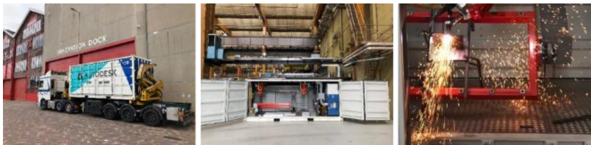
Example of a mobile WAAM system (developed by Valk Welding and owned by Autodesk): shown during transportation (left); installed and ready for operation (centre) and during operation (right).
