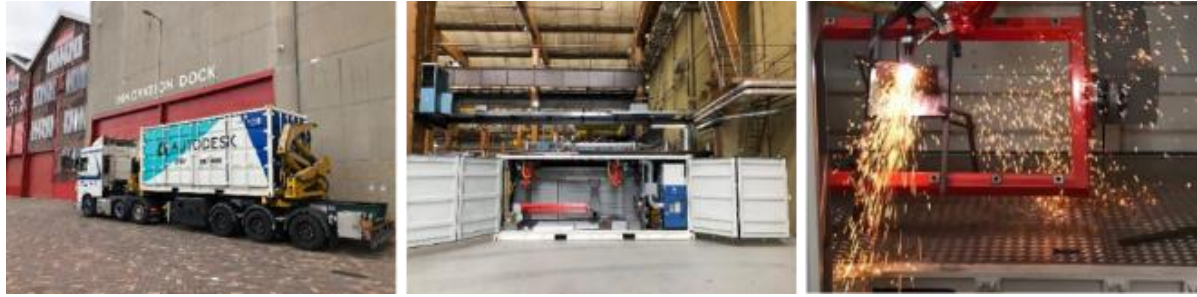
Figure 6. Example of a mobile WAAM system (developed by Valk Welding and owned by Autodesk): shown during transportation (left); installed and ready for operation (centre) and during operation (right).
