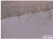
Interface AM410 to CuAl8 indicating 1st to 4th deposit of CuAl8, indications of liquid metal embrittlement and cracks, inhomogeneous mixing at the interface
