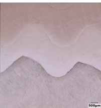
Micrograph between AM46 and AM410, indicating several layers of AM410
