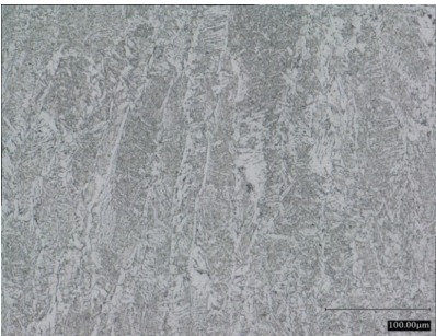
micrographs AM35 a) Columnar solidification structure b) fine grained heat affected zone
