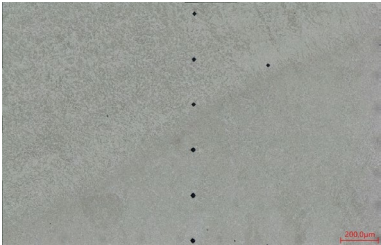
Micrograph of fusion line between first and final layer of Fe-Fe2. Hardness Vickers indents are seen
