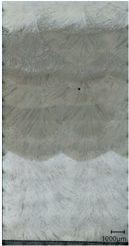
Macrograph bottom layers LNM MoNi , top layers LNM 4M (Fe-Fe2)
