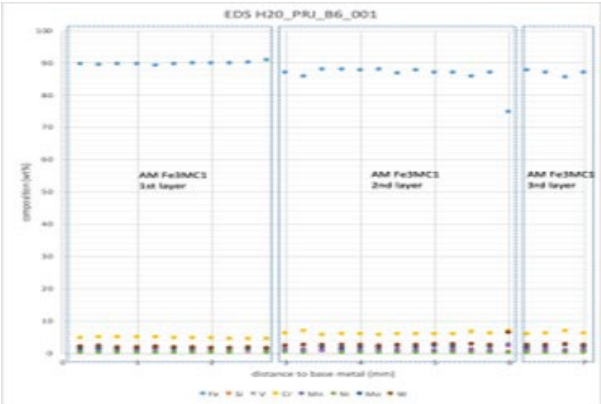
Composition along building direction from 1st layer of Fe3MC1 (TUD)
