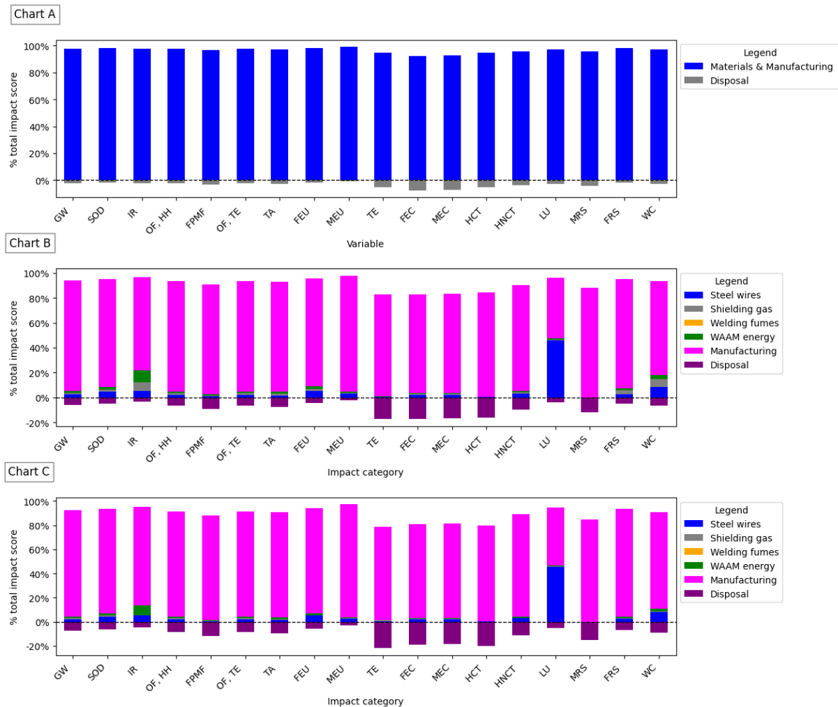
Figure 26. Process contribution of Gorenje Orodjarna demonstrator B-4.1 produced with (A) conventional manufacturing; (B) WAAM (worst) and (C) WAAM (best). By looking at (A) the materials&manufacturing life cycle stage is the most contributing process. The major difference between WAAM (best) and WAAM (worst) is the contribution of shielding gas to the total impact score which appears in Ionizing radiation and Water consumptions categories when WAAM (worst) is considered. The most contributing process in manufacturing except for Land use that is the steel wire production. For all scenarios it is possible to notice a negative contribution of the recycled material to the total environmental impact, this is due to crediting in the system modelling. This is based on characterized results calculated with ReCiPe2016 (H) without Monte Carlo analysis.
