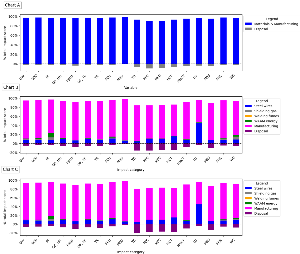
Figure 30. Process contribution of Gorenje Orodjarna demonstrator B-4.2 produced with (A) conventional manufacturing; (B) WAAM (worst) and (C) WAAM (best). By looking at (A) the materials & manufacturing life cycle stage is the most contributing process. There are no evident differences between WAAM (best) and WAAM (worst). The most contributing process in manufacturing except for Land use that is the steel wire production. The major difference between WAAM (best) and WAAM (worst) is the contribution of shielding gas to the total impact score which appears in Ionizing radiation and Water consumptions categories when WAAM (worst) is considered. For all scenarios it is possible to notice a negative contribution of the recycled material to the total environmental impact, this is due to crediting in the system modelling. This is based on characterized results calculated with ReCiPe2016 (H) without Monte Carlo analysis.
