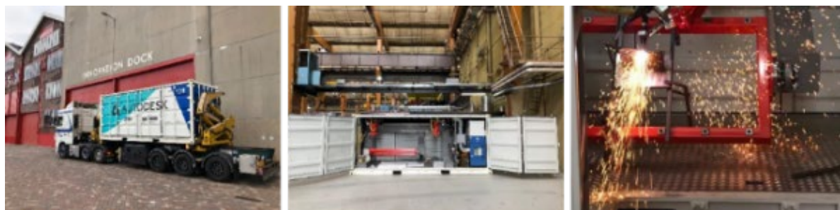
Pictures above: Example of a mobile WAAM system (developed by Valk Welding and owned by Autodesk): shown during transportation (left); installed and ready for operation (centre) and during operation (right).
